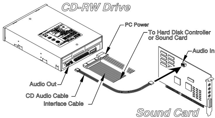
5. If you have a sound card that can be connected to this CD-ReWritable drive, you can connect the drive (as Audio-out) and the sound card (as Audio-in) with a 4-pin audio cable. (See figure above.)
